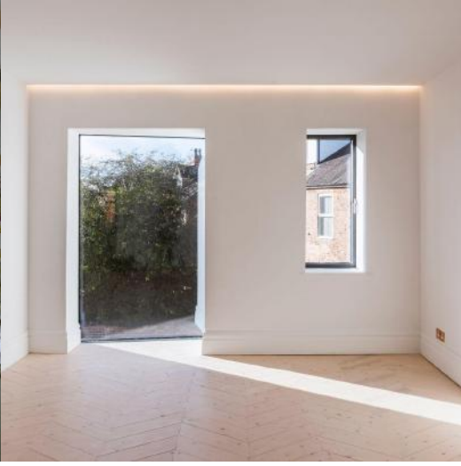
Twisting the West facing glazing on the first floor further to the south within the construction build up was modelled to show a 15% increase in the amount of solar gains.
